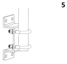
INSERT THE POLE INTO THE U-BOLTS AND TIGHTEN.
